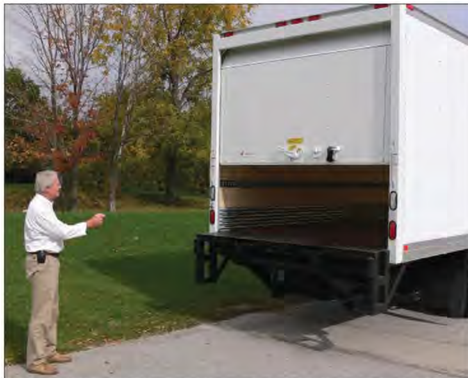
EASY TO USE: The roll-up door on this straight truck is opened with the click of a button, using the handheld keychain-type remote control.
