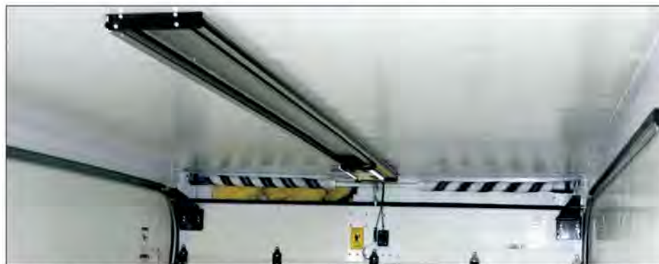
BRIGHT IDEA: The interior LED lights travel along the track on the ceiling so they're not blocked by the door when opened.
